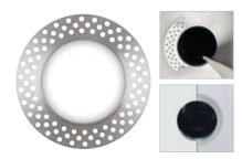
**Mud-in ring (FT):** Low profile, machined aluminum mud-in ring provides a raised rib to plaster up to and a 3/16" flange thickness. The ring is attached to the ceiling material as opposed to the frame-in kit to avoid conduction of heat and vibration which can cause yellowing or cracking of the plaster.
