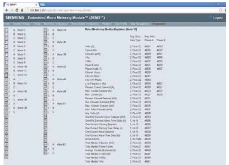
Diagnostics: Displays all active metering and can provide metering Modbus Register information
