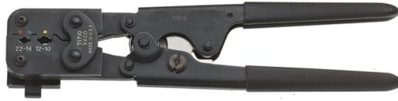
Compound-action tool crimps 10-22 AWG insulated terminals to meet or exceed MIL-SPEC pull-out tests. Built-in ratchet with safety release ensures uniform crimps every time. Compound lever-action of narrow-span handles puts more crimping power into each squeeze.
