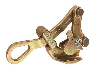
Lightweight, compact grips pull an exceptionally wide range of cable sizes and types. Designed with a round inside-jaw contour for maximum contact to minimize conductor damage. Lower jaw is serrated to firmly grip insulated cables and conductors. Design includes a latch that prevents the grip from falling in case of jaw disengagement from the cable.
