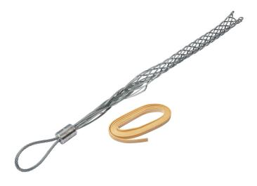
These medium-duty, standard length double-weave split mesh wire pulling grips from Klein combine strength and durability for to help linemen get the job done. Manufactured, inspected and test in the USA, these grips are made of drop-forged quality US steel. Grips are rigorously tested using the Magnuflux method and pulled to rated load to ensure the highest quality and reliability.
