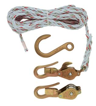
All Klein block and tackle use high-quality, 3/8" (10 mm) diameter rope. Light, galvanized-steel shell blocks are fitted with snubbing hooks to hold the load. This package features two blocks with an anchor hook with a maximum safe load is 750 lbs. (340 kg).
