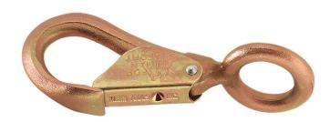
The Klein Tools Snap Hook easily connects to rope for hoisting. Manufactured with forged steel and features a quick-acting plunger-style hatch. Maximum safe load 1500-pounds (680 kg).
