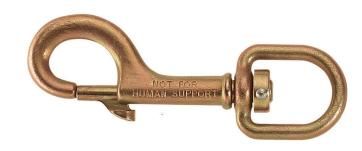
The Klein Tools 750-pound 1/2-Inch Steel Swivel Hook with Plunger Latch is made from forged steel. It can hold up to 750 pounds. The swivel action of the clevis allows smooth rotation to help prevent accidental fouling into secondary wires.
