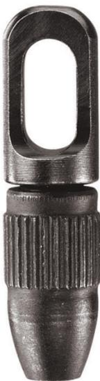
For use with 1/8-Inch (3 mm) wide steel fish tapes. The swivel head design helps prevent kinks and allows smoother, easier fishing in tight turns. High capacity eyelet holds up to five #12 unstripped wires or seven #10 bare wires.
