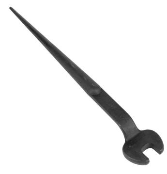
Forged from select alloy steel, the Klein Tools 3/4-Inch Nominal Opening Spud Wrench is designed to withstand high-leverage and heavy loads. It's designed for use with 1/2-Inch bolts and U.S. regular nut types. The extra-duty head area gives maximum strength and durability. Plus, the continuous taper of the handle makes it easy to line up bolt holes.
