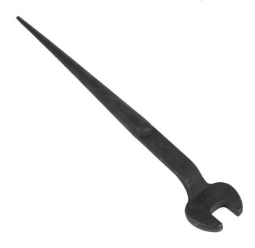
Forged from select alloy steel, the Klein Tools 13/16-Inch Nominal Opening Spud Wrench is designed to withstand high-leverage and heavy loads. It's designed for use with 1/2-Inch bolts and U.S. regular nut types. The extra-duty head area gives maximum strength and durability. Plus, the continuous taper of the handle makes it easy to line up bolt holes.
