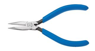
These lightweight, slim long-nose pliers feature polished inside jaws with radiused edges to prevent nicking of wire during delicate assembly work. Curved handles provide greater tool control. This pair is spring-loaded for self-opening action. Made of forged steel for maximum durability and long life.
