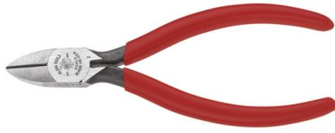
These 5-Inch Diagonal Cutting Pliers have a tapered nose to easily work in confined areas and allow close tip cutting. They come with short jaws and beveled standard cutting edges to permit close wire cuts. The pliers are forged from US-made steel and have induction hardened knives and a hot-riveted joint for a long lasting smooth action.
