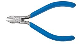
These Electronics Pliers are the smallest diagonal-cutter Klein offers for close quarter work. They feature a miniature jaw for maximum visibility in tight spaces. The sharp, pointed, tapered nose allows for precise tip cutting. The short jaws and semi-flush, beveled cutting knives permit close cutting of wire. Made of the finest U.S. steel alloy and induction hardened for long life.
