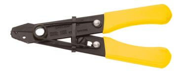
Klein Tools 1004 Wire Stripper and Cutter is a handy, light, compact tool for stripping insulation. Spring-loaded for action for self-opening. Convenient hole for looping or bending wire. Adjustable slide stop with set screw for repeat stripping work.
