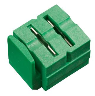
Designed for use with Klein's Radial Strippers. Two levels of blades strip mini coaxial cable. Pre-set cutting blades for precise and accurate stripping. Durable high-carbon steel cutting blades are ground and honed for long life. Patented "V" notch eliminates scoring of the center conductor.
