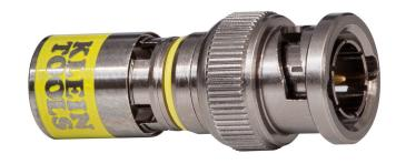
Klein's patented universal sleeve technology BNC connectors install up to 5x faster than other BNC compression connectors. Patented viewing windows in sleeve aid in proper seating. One connector fits all diameter variations within a cable series. This patented sleeve design provides the excellent holding power and signal strength you demand.
