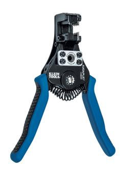
Klein Tools' Katapult® Solid and Stranded Wire Stripper / Cutter has a built-in cutting hole to cleanly cut 8-20 AWG solid and 10-22 AWG stranded wire, while the stripping head allows you to easily grip and strip just by squeezing the handle. Made of cast alloy with a heavy-duty Ecoat finish for corrosion resistance and durability.
