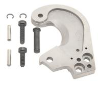
This replacement blade set for the Ratcheting ACSR Cable Cutter (63607) cut copper, aluminum and ACSR. Forged, heat-treated, shear-type cutting blades are made of hardened steel for sharpness and long life.
