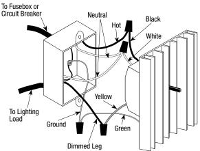
Figure B.Wiring Diagram
