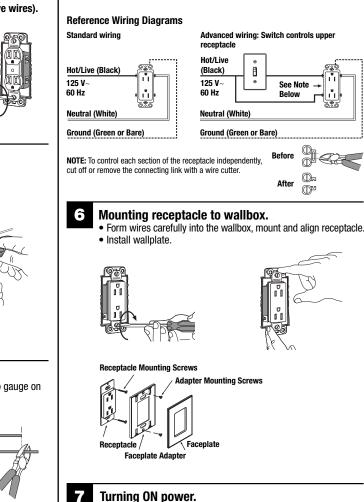
Turn power ON at circuit breaker (or replace fuse).
