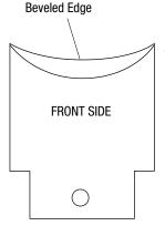
3. Use a high-speed dremeltype tool to flatten top edge of blade (approximately 1/32" wide flat).
