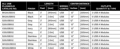
Available in 5' [1.5m] length with 9" spacing. 15A tamper-resistant receptacles. 3-wire, #12 THHN (1 hot, 1 neutral, and insulated ground conductor rated for use on 20A circuits). .040" [1.0 mm] steel housing. Packed two per carton. Each unit supplied with one (1) Coupling and two (2) Blank End Fittings. USB is 2.4 Amps (shared between two ports) 5VDC. Please note the charging load on one module will not affect the charging performance of the other USB modules in the product.
