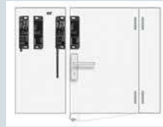
Non-contact safety magnetically operated switches (with plug or cable) for right-hinged door
