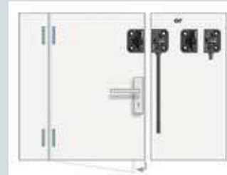
Non-contact safety magnetically operated switches (with plug or cable) for left-hinged door
