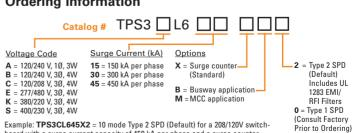
board with a surge current capacity of 450 kA per phase and a surge counter.
