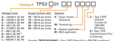
Example: TPS3C0120X002 = Type 2 SPD (Default) for a 208/120V panelboard = 400/230 V, 3Ø, 4W with a surge current capacity of 200 kA per phase and a surge counter. When an option is not selected, include a zero (0) in the field.
