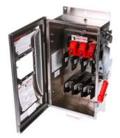
Siemens Low Voltage Circuit Protection Heavy Duty Safety Switches. Type: ENCLOSED, SAFETY SWITCH Std: CSA V. Rating: 600V A. Rating: 200A Wattage: 3W No. Of Poles: 3P F. Rating: 60Hz Action: SINGLE THROW Material: SS Enclosure: TYPE 4X. 2-3 point mounting holes. Insulation: YES O. Cycles: 8000 O. Temperature: (-20F-120F) AMBIENT TEMPERATURE Environmental Conditions: INDUSTRIAL CORROSIVE RESISTANCE
