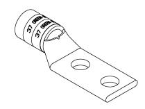
WIRE SIZE: #1 AWG MATERIAL: HIGH CONDUCTIVITY COPPER
