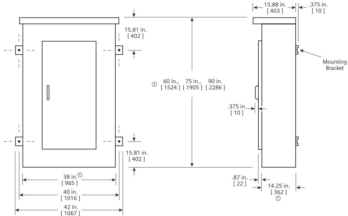
①Dimensions are interior of the box. Add 5/8" to width for absolute dimension. Add 1/8" to height for absolute dimension.
