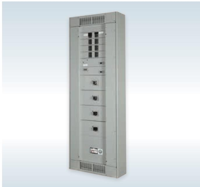
The P5 panel configurations defined by the unit space allowed for a given amperage, main device and box height. The P5 panel starts with a 60" high box. All of the branch devices are unit space mounted. Breakers and switches can be mixed and matched to meet customer requirements.
