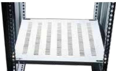
Vented Frame Shelf mounts to the vertical hole pattern on a frame and provides a stationary surface for equipment. The shelf is 16 gauge steel finished with RAL 7035 textured gray polyester powder paint.
