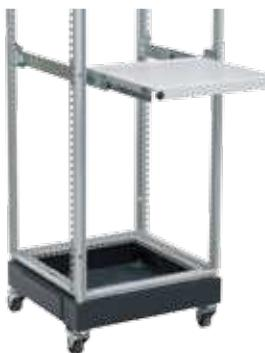
Frame Pull-Out Shelf allows easy access to shelf-mounted devices. The shelf is 16 gauge steel with 12 gauge steel supports. The entire assembly is finished with RAL 7035 textured gray polyester powder paint. The shelf mounts to the front and rear frame uprights. Load rating is 110 lb. (50 kg).
