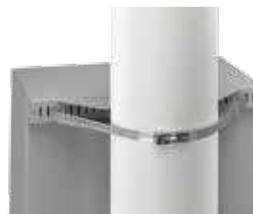
Enable COMLINE, CONCEPT, ACCESSPLUS, D-BOX and L-BOX enclosures to be mounted to poles of various sizes and shapes. Simply attach the galvanized steel channel bar to the mounting holes at the back of the enclosure, then wrap the stainless steel strap around the pole and through the bar. Kit includes two mounting channels, two straps suitable for up to 12-in. diameter pole, and mounting hardware.
