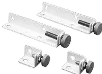
Provide additional support for panels on which heavy components are mounted. Each panel support fits over a collar stud and is then adjusted so the weight of the panel is partially supported by the bottom of the enclosure. Locknuts prevent accidental change in adjustment. A polyethylene-covered base on each panel support distributes the panel weight and prevents damage to the interior finish. Constructed of heavy-gauge steel. White finish.
