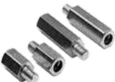
Threaded Panel Extenders are made of plated steel and designed to raise the panel mounting surface. Extenders attach to threaded internal pads. Male and female thread size is 10-32. Each kit contains 4 extenders.
