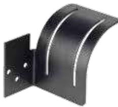
Provides support for cable in transitions between horizontal and vertical routing. Mounts to strut, grid strap or PROLINE and Network Vertical Tie-Down Cable Managers. Can be used with VELCRO® Cable Wrap (order separately). Made of steel coated with RAL 9005 black polyester powder paint. Includes mounting hardware.
