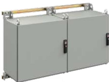
The PROLINE G2 Anti-Tip Bracket Kit secures the top of an enclosure to a fixed surface such as a wall, and protects against enclosure tipping. The brackets are made from 10 gauge mild steel, and are Polyester powder-painted RAL 7035 textured light gray. The kit comes with a single pair of brackets and mounting hardware to affix brackets to the enclosure.
