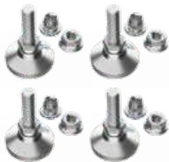
The Post-type Leveler Kit allows for height adjustment at the enclosure corners to account for uneven floors. Levelers thread into the frame corners, and can be used with a bottom-mounted Gland Plate or a 0-mm Solid Base; they may also be affixed to the corner blocks of the standard Plinth Base. Levelers are plated for indoor use, and are rated to 3000lbs (1361kg).
