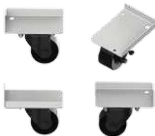
The Plate Caster Kit consists of four polyamide casters (two locking and two non-locking) secured to formed-steel plates painted RAL 7035. The Plate Caster hardware secures the caster at the frame corners, and can be used with a bottom-mounted Gland Plate or a 0-mm Solid Base; however, they do not work with Plinth Bases. Plate Casters can also be used on joined PROLINE G2 enclosures,
