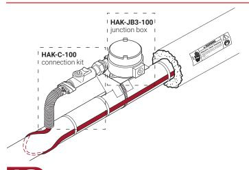
The nVent RAYCHEM HAK-C-100 connection system is FM approved for use with nVent RAYCHEM HBTV, HQTV, HXTV, and FHP heating cables in Class I, Division 1 hazardous locations. It is also CSA certified for use with nVent RAYCHEM BTV-CT, QTVR-CT, XTV-CT, VPL-CT, and LBTV2-CT heating cables and c FM us approved for use with nVent RAYCHEM HTV heating cables in Class I, Division 1 locations.
