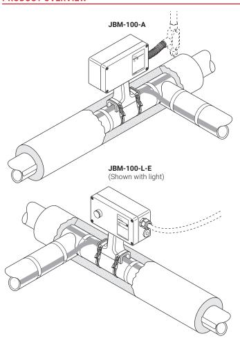
The nVent RAYCHEM JBM-100 kit serves as a power connection, splice, or tee for up to three nVent RAYCHEM brand BTV, QTVR, XTV, KTV, HTV or VPL heating cables. It is approved by FM, CSA, PTB and IEx for use in hazardous locations.
