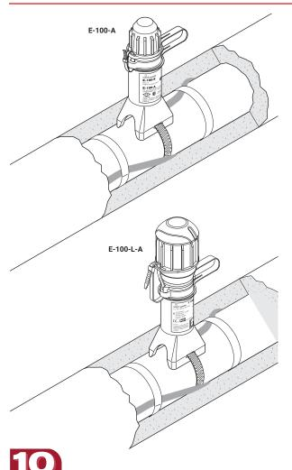
The nVent RAYCHEM E-100-A and E-100-L-A serve as above-insulation end seal kits for nVent RAYCHEM brand BTV, QTVR, XTV, KTV, HTV or VPL heating cables. They are approved for use in hazardous locations.
