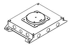
RFBA 4-Gang Round Floor Box, Shallow 3.25" Depth - Steel floor box designed for above grade installations. Features 4-gangs of box capacity with at least 2 %6" available behind device plates. Fully adjustable before and after concrete pour. Designed for carpet, wood flooring, tile, terrazzo and polished concrete applications. Use with Evolution™ Series 6" round covers.
