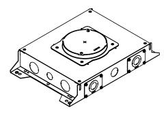
RFBA 4-Gang Round Floor Box, Standard 3.75" Depth - Steel floor box designed for above grade installations. Features 4-gangs of box capacity with at least 2 %6" available behind device plates. Fully adjustable before and after concrete pour. Designed for carpet, wood flooring, tile, terrazzo and polished concrete applications. Use with Evolution™ Series 6" round covers.
