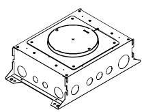
RFBA 10-Gang Round On-Grade Floor Box, 6.25" Depth - Steel floor box designed for on-grade installations with a fusion-bonded epoxy for use on metal reinforcement bar and related accessories before encapsulating in concrete. Features 10-gangs of box capacity with at least 2 ½" available behind device plates. Fully adjustable before and after concrete pour. Designed for carpet, wood flooring, tile, terrazzoand polished concrete applications. Use with Evolution™ Series 8" round covers.
