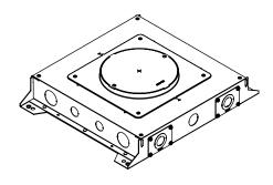
RFBA 6-Gang Round Floor Box, Standard 3.75" Depth - Steel floor box designed for above grade installations. Features 6-gangs of box capacity with at least 2 %6" available behind device plates. Fully adjustable before and after concrete pour. Designed for carpet, wood flooring, tile, terrazzo and polished concrete applications. Use with Evolution™ Series 8" round covers.
