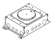
RFBA 10-Gang Round Floor Box, 6.25" Depth - Steel floor box designed for above grade installations. Features 10-gangs of box capacity with at least 2 ½" available behind device plates. Fully adjustable before and after concrete pour. Designed for carpet, wood flooring, tile, terrazzo and polished concrete applications. Use with Evolution™ Series 8" round covers.
