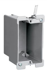
Durable, impact-resistant thermoplastic box complemented by innovative extras that cut installation time. Single Gang, Old Work Switch and Outlet Box with Swing-Bracket for mounting. Adjusts from 1 1/4" down to 1/8". Two Auto/Clamps on Each End. 100 pack.
