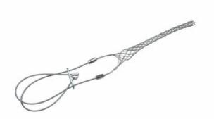
Bus drop, Closed mesh, Locking bale. Cable diameter - 15-inch, Bale length - 6.5-inch, Mesh length - Break strength 1,100 lbs.
