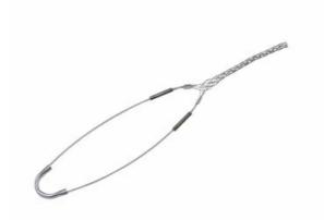
Bus drop, Closed mesh , Single eye. Cable diameter - 0.220-0.320-inch, Bale length - 9-inch, Mesh length - 3.5-inch, Break strength - 1,100 lbs.
