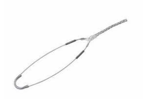
Bus drop, Closed mesh, Single eye. Cable diameter - 0.700-0.850-inch, Bale length - 9-inch, Mesh length - 8.5-inch, Break strength - 1,900 lbs.
