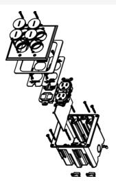
Wiremold WMFB2DRKS4B Series Dual-Gang Floor Box Assembly Part No. WMFB2DRKS4B
