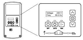
The RDC2 controller provides integrated control for the generator set, Kohler<sup>®</sup> Model RXT transfer switch, programmable interface module (PIM), and load management device.
