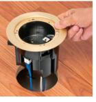
4 Place floor box into hole. Orient as desired. Tighten wing screws to secure box to floor.
