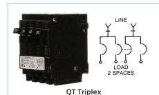
These space saver triplex breakers provide a 2-pole common trip breaker for 120/240V AC circuits and two single poles for 120V AC circuits. Triplex require two panel spaces. HACR rated.
