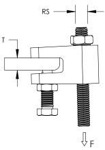
nVent CADDY Rod Lock beam clamp not for use with hot dip galvanized threaded rod. \*CRLB37EG and CRLBM10EG Beam Clamps are listed per UL 2239 and UL 203 in method #1 & #2 orientations. \*\*CRLBM8EG is listed per UL 2239 only in method #1 & #2 orientations.
