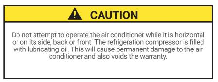
TEST FOR FUNCTIONALITY BEFORE MOUNTING THE AIR CONDITIONER TO THE ENCLOSURE.
