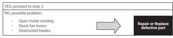
3. Check thermostat setting and adjust thermostat to the lowest setting. This should turn the condenser fan and the compressor on. Did condenser fan and compressor come on when the thermostat was turned on?
