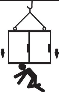
Loose fasteners can cause cabinet(s) to fall and cause serious injury or death and product damage.
