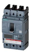
circuit breaker 3VA6 UL frame 150 breaking capacity class M 35kA @ 480V 3-pole, line protection ETU550, LSI, In=150A overload protection Ir=60A...150A short-circuit protection Isd=0.6..10x In, Ii=1.5..10x In N conductor protection optionally with external current transformer, up to 160% without connection
